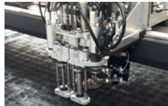
Double hollow punch device from 5 to 25mm diameter.
