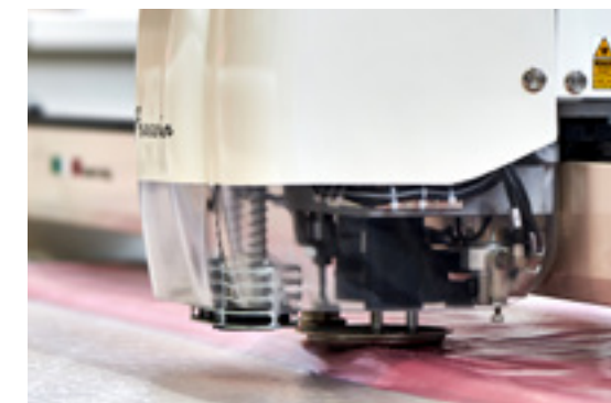
Single or double drilling device with temperature control.
