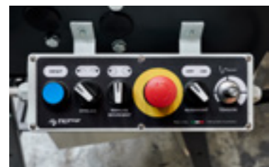
Control panel allowing any actions in order to feed, rewind, stop, start, align, etc.
